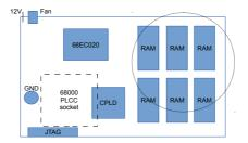
Due to space restrictions, Ninetails is not compatible with standard Amiga 600 hard disk mounting cradle. It is advised to use Compact Flash instead of hard disk.
